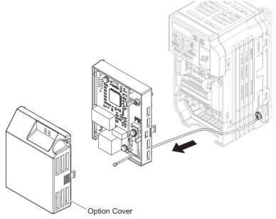
Figure 15 Ground Wire Routing
