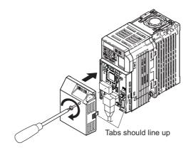
Figure 20 Attach the Option Cover
