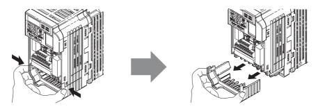
Figure 5 Remove the Bottom Cover on an IP20/Open-Chassis Drive (Models CIMR-V□BA0001B to BA0003B and 2A0001B to 2A0006B)
