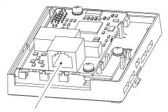
Figure 18 Communication Cable Port
